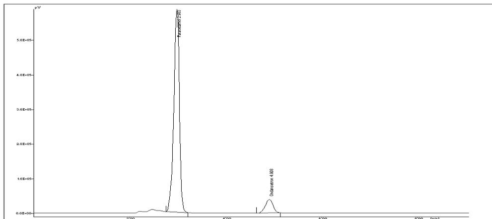
Fig. 4. Chromatogram of OND ( $t_R$  4.8 min) and PARA ( $t_R$  2.9 min) of formulation (ONDEM-P) showing no interference of excipients in analysis.
