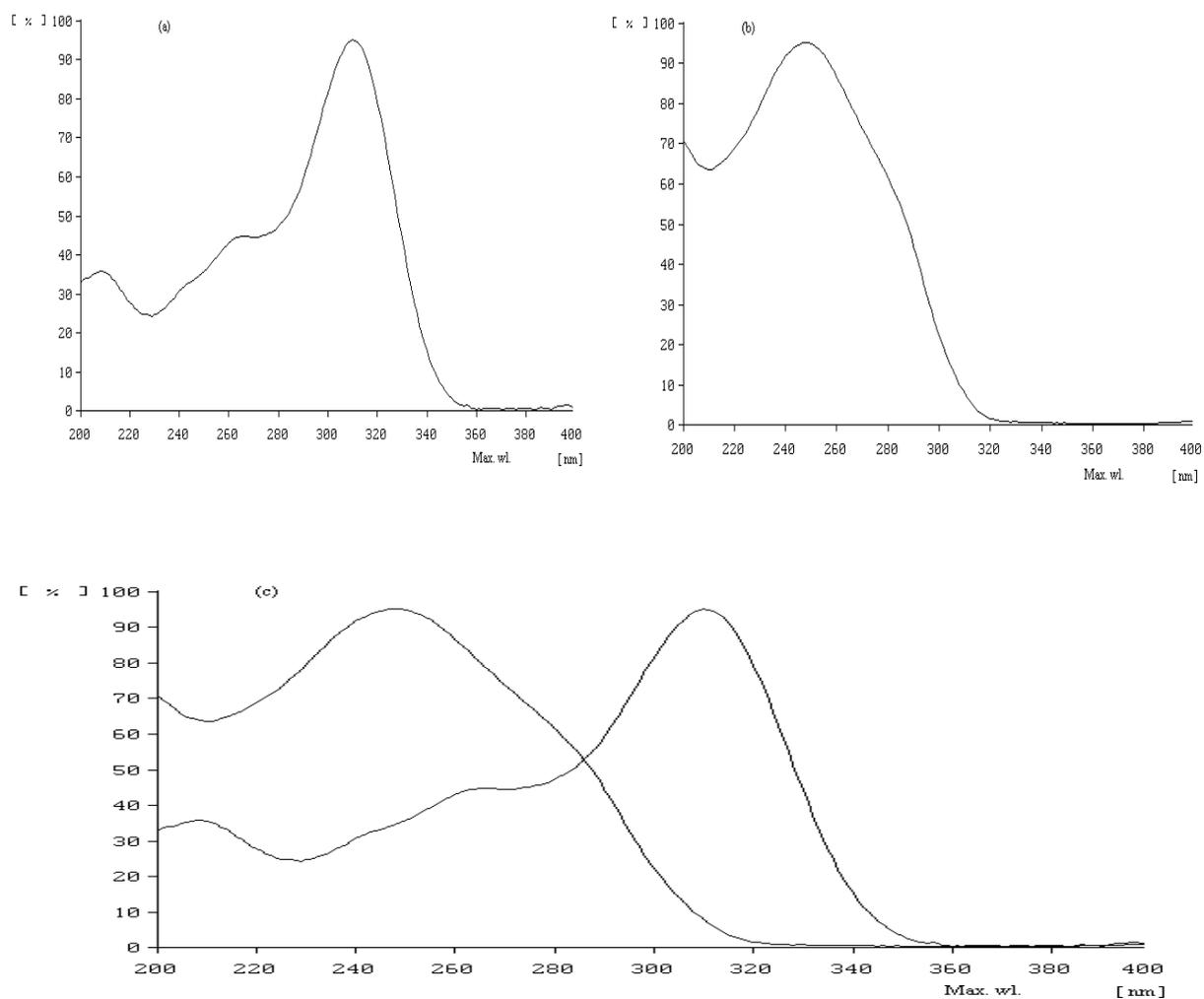
Fig 2 Representative spectrum of (a) OND, (b) PARA, (c) In-situ overlain spectrum of OND and PARA.
