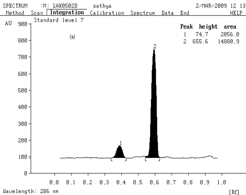
Fig. 5 Densitogram of OND ( $R_F$  0.39) and PARA ( $R_F$  0.59) of formulation (ONDEM-P) showing no interference of excipients in analysis.
