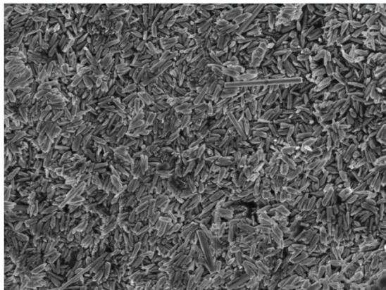
**Figure 2. SEM microphotograph of fabricated silver nanoparticles.**
